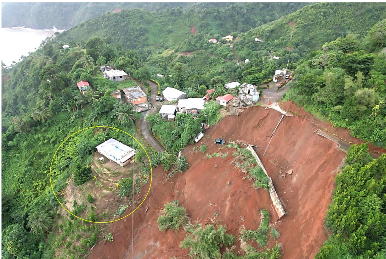
Kent Copiel, IICA Technical Specialist in Dominica pointed out the vetiver hedgerows (encircled in yellow) recently planted on the slope by the EbA project team, unaffected by the landslides which followed a true ridge-to-reef flow, as it made its way all the way down to the coast. (Photo: Amos Benjamin)
